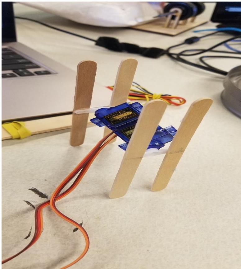
The first iteration failed to work. One of the initial barriers I came across was that 0 degrees were not exactly the same on each motor, since you could remove and replace the head of the motor. Furthermore, vibrating the motors did not cause it to
