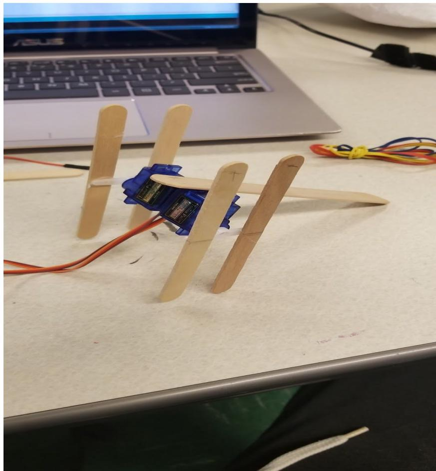
The second iteration added a tail to the robot. This did help a little, but it became quite obvious that the design would not be functional as intended. The weight of the tail seemed to be too much, and, if it did move at all, it would move in the direction of the tail or in a circle. This is not the point of a tail. I also added the +/- on the popsicle sticks in order to ensure I did not confuse how the motors were orientated, as was a problem in the first prototype.
